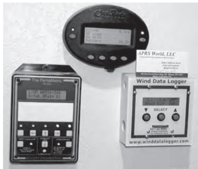
Christian Milaster's "cockpit" which measures wind energy, electricity consumption and conversion from DC to AC current.
